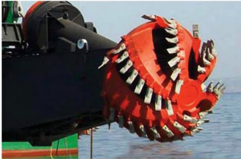
SUCTION HOSE FITTED TO 34 - 36 - IINCH - DREDGE - CUTTER HEAD
